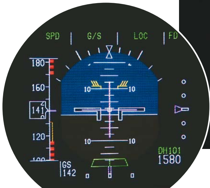
Below: Boeing 757 Electronic Attitude Direction Indicator, speed tape showing 141 kt IAS, groundspeed 142, RadAlt 1,580 ft and decision height 101 – on centreline and on glidepath too!
