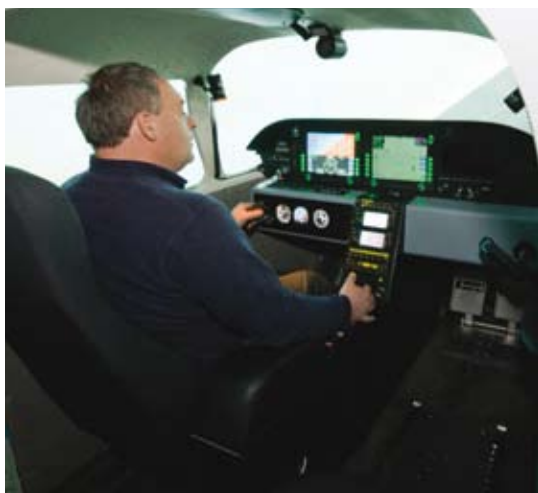
Procedural trainers such as this Cirrus trainer give GA pilots a chance to simulate problems without taking to the air
